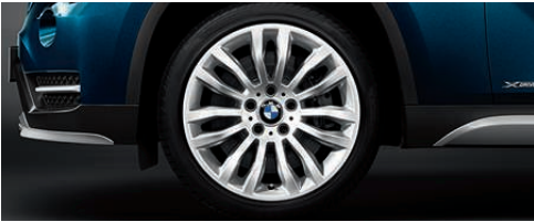
□ 18" light alloy wheels Double-style 321 , 8 J x 18 with 225/45 R 18 runflat tyres.
