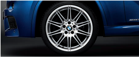
□ 19" M light alloy wheels Double-spoke 225 M with mixed runflat tyres, front 8 J x 19 with 225/40 R 19 tyres, rear 9 J x 19 with 255/35 R 19 tyres (exclusively available with the M Sport package).
