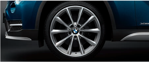
□ 19" light alloy wheels V-spoke 324 with mixed runflat tyres, front 8 J x 19 with 225/40 R 19 tyres, rear 9 J x 19 with 255/35 R 19 tyres.
