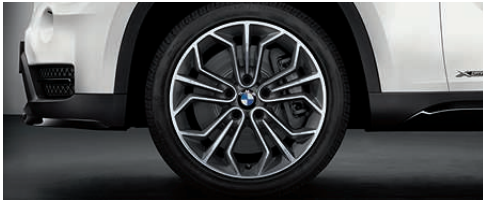
□ 18" light alloy wheels Honeycomb spoke style 323 , bi-colour, with mixed runflat tyres, front 8 J x 18 with 225/45 R 18 tyres, rear 9 J x 18 with 255/40 R 18 tyres.
