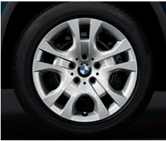
■ 17" steel wheels with wheel covers 1 , 7.5 J x 17 with 225/50 R 17 tyres, also available as a complete winter wheel set from the Original BMW Accessories range (standard with X1 sDrive16d, X1 sDrive18i, X1 sDrive18d, X1 xDrive18d).
