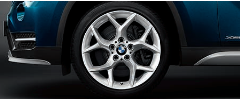
□ 18" light alloy wheels Y-spoke 322 , 8 J x 18 with 225/45 R 18 runflat tyres (exclusively available with xLine).
